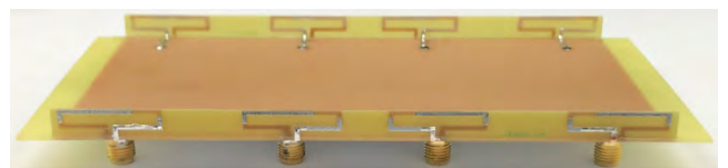
FIGURE 15. Photo of the fabricated antenna prototype of 8-antenna MIMO system with L1 = 22 mm, L2 = 21.5 mm, and d23 = 10 mm.
