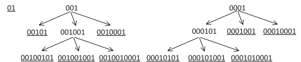
FIGURE 2. Partial extensions over the minimal set \{01, 001, 0001\} . Underlined codewords are in the final set after partial extensions.
