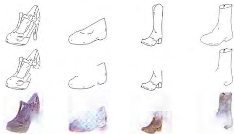
FIGURE 2. cGAN based image-to-image translation applied to incomplete images (Top: Complete sketches given as references, Middle: Incomplete sketches given as input images, Bottom: Translated output images). Notice that the translated output images inherit the missing parts of the given input sketches.
