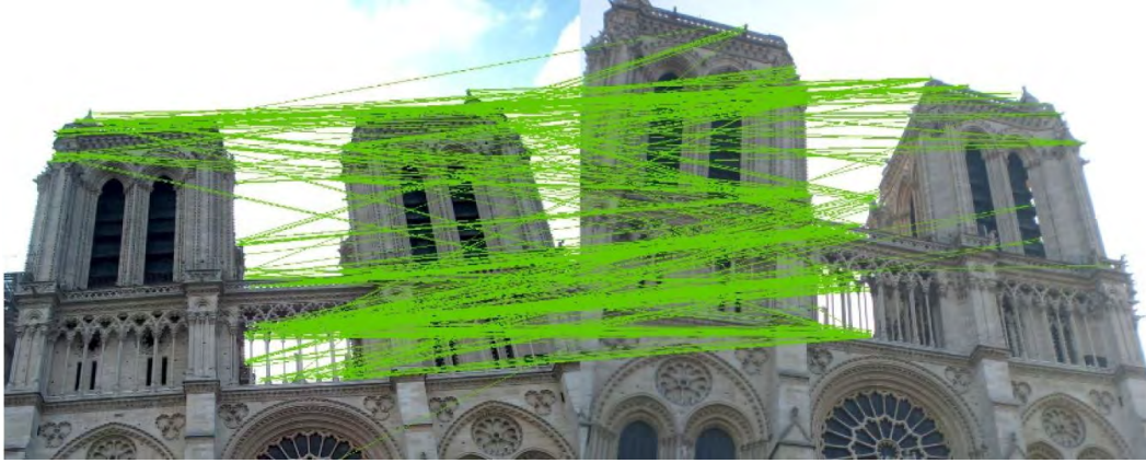
FIGURE 2. Visual correspondences of two views with repeated features, rotation and illumination variation, where some incorrect matches are produced.
