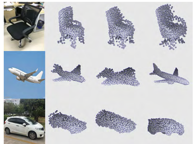
FIGURE 12. Each method occupies one column, the first column is the 2D image, and the three methods are PSGN, simplified RealPoint3D and RealPoint3D.
