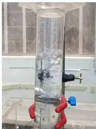
FIGURE 5. Phenomenon of water displacement through gas evolution under 20 A after 1.5 h DC in saturated coke.
