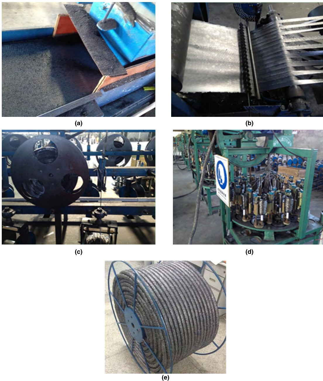
FIGURE 1. Pictures of the actual productive process. (a) Rolling of the graphite paper. (b) Cutting into slim. (c) Twisting into the graphite wire. (d) Weaving into the graphite grounding material. (e) The finished flexible graphite grounding material.
