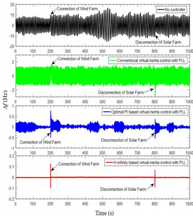
**FIGURE 12.** Frequency response under high RESs penetration.
