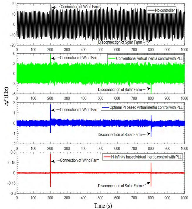
**FIGURE 13.** Frequency response under severe system uncertainties.
