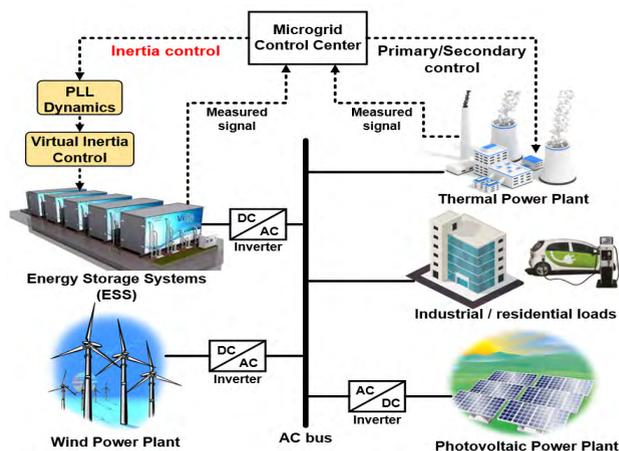
FIGURE 1. A schematic diagram of the islanded microgrid.
