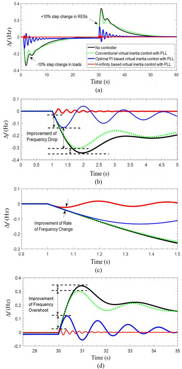
**FIGURE 10.** Microgrid response: (a) Frequency stability under sudden load/RESs changes. (b) Improvement of system frequency drop. (c) Improvement of ROCOF. (d) Improvement of system frequency overshoot.
