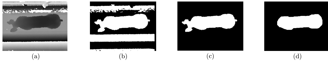
FIGURE 4. The image processing procedure: (a) the grayscale Kinect depth image before processing, (b) the image after conversion to binary with an appropriate threshold, (c) the binary image after removing all but the largest connected object, and (d) the binary image after erosion and dilation.
