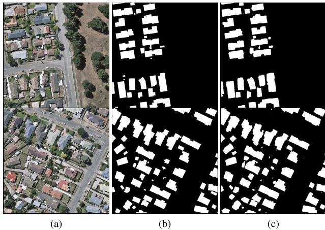
FIGURE 1. Examples of building extraction. (a) Aerial images. (b) Ground truth in which buildings are in white and background is in black. (c) Prediction of our network.
