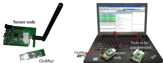
FIGURE 9. Sensor node, grabber and platform of experiments.
