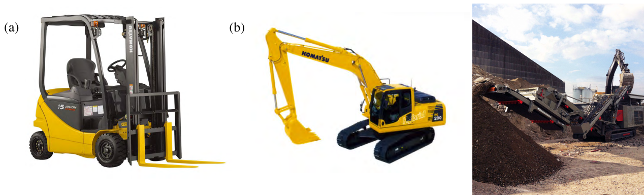
FIGURE 19. Industrial machines that use SCs. FB15HB-12 battery – SC hybrid forklift for Komatsu (a), PC200–8 Hybrid Excavator (b) and Rockster R1100DE Parallel Hybrid Crusher (c). Photos taken from the manufacturers websites.
