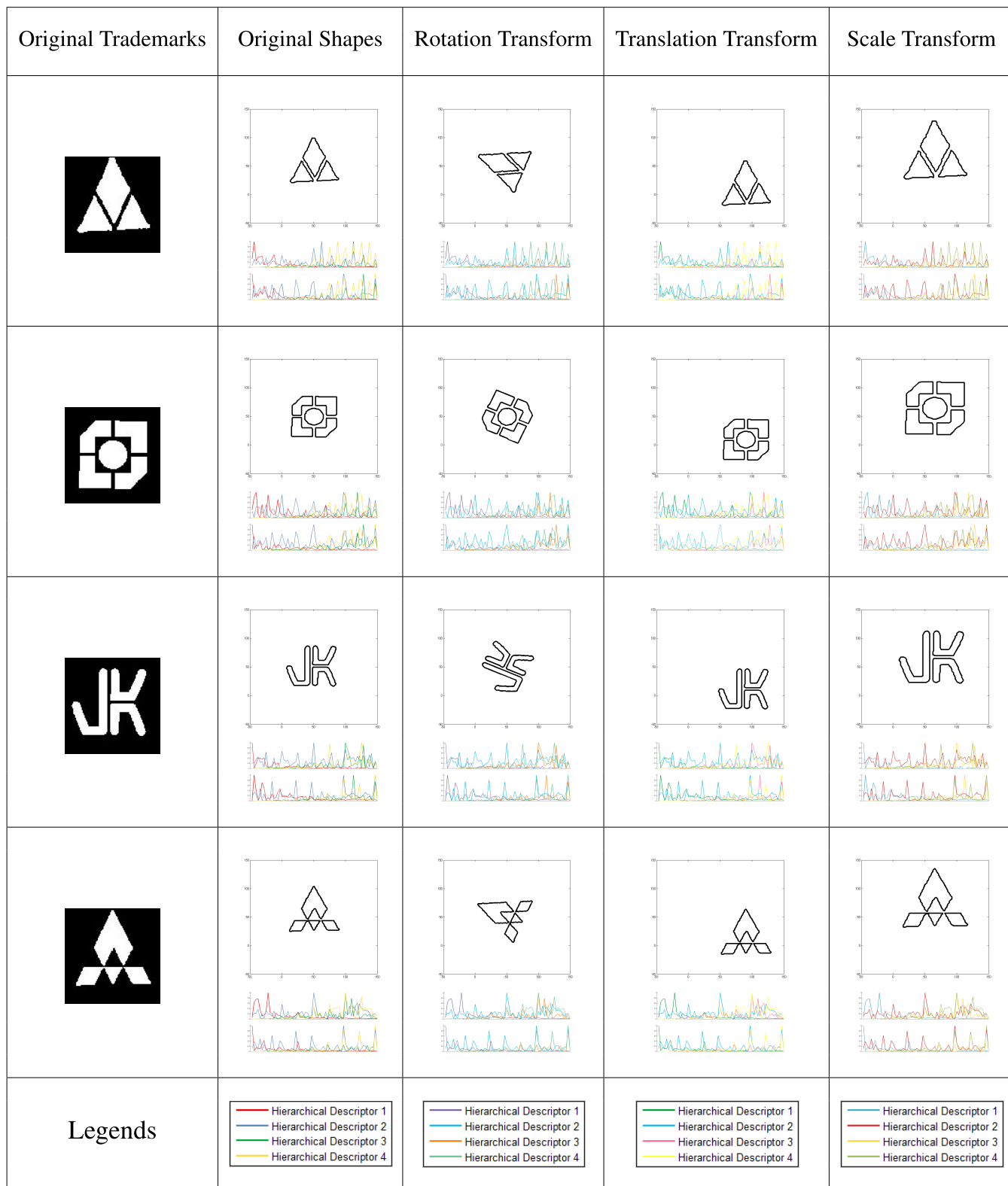
FIGURE 8. The invariance experiments of hierarchical V-system descriptors. Four examples with regular complex trademark and irregular complex trademark, the results contains the original, rotate, translation, and scale transform shape and their energy frequency descriptors of x and y .
