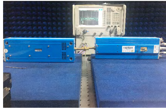
FIGURE 8. Measurement setup for the W-band extraction.
