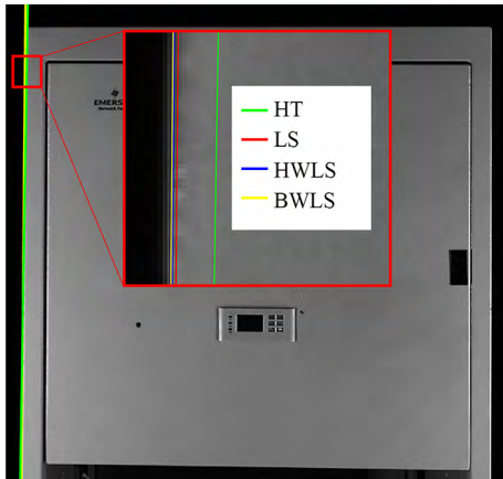
FIGURE 7. Fitting lines obtained with the HT, the LS, the HWLS, and the BWLS algorithms.
