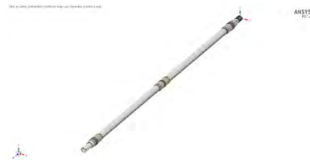
FIGURE 10. Model 1: add a centralizer bearing in the middle part of the most easily deformed shaft.
