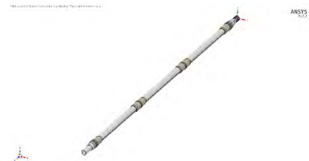
FIGURE 11. Model 2: add two centralizer bearings at the full length of the 1/3 from the two ends of the shaft.
