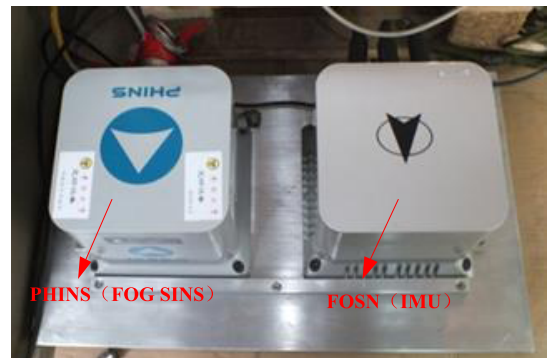
FIGURE 14. Installation of the vehicle simulation experiment equipment.
