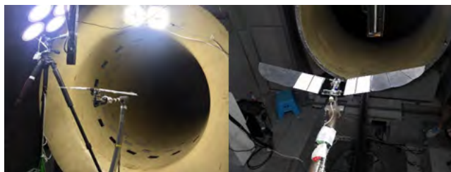
FIGURE 3. Installation of the experimental system in the wind tunnel.
