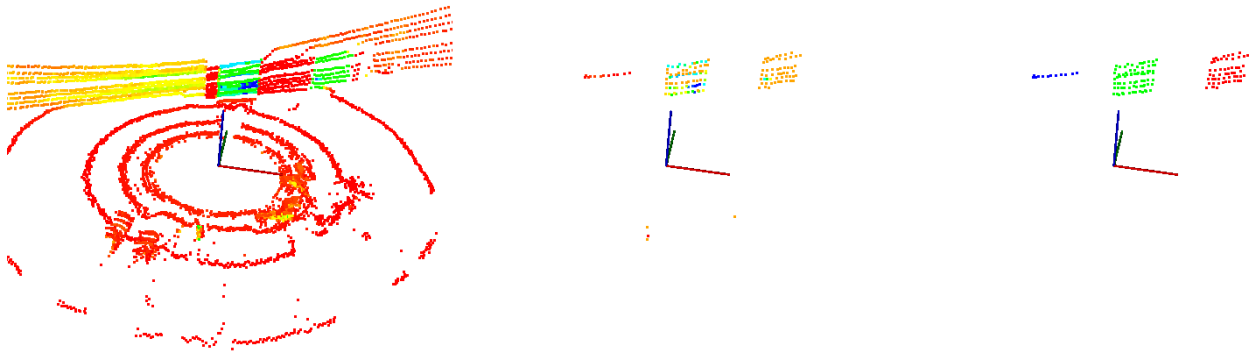
FIGURE 3. Reflective beacon in point cloud (left, color represents intensity), intensity filtered and down-sampled point cloud (middle, color represents intensity), and cluster extraction (right, color changes represent different clusters).
