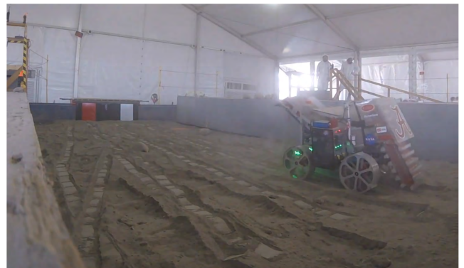
FIGURE 11. Robot navigating autonomously with localization system (beacon is against the back wall).
