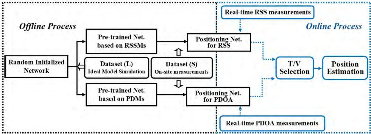
FIGURE 3. Flowchart of the selection based hybrid ANN-PDOA and ANN-RSS positioning system with pre-training.
