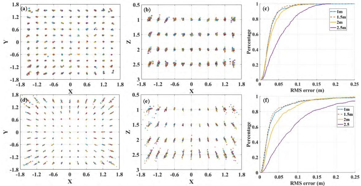
FIGURE 12. ANN-PDOA and ANN-RSS performances' comparisons with no intensity variations a) X-Y view of ANN-RSS positioning results; b) X-Z view of ANN-RSS positioning results; c) RMS error CDF of ANN-RSS positioning at different heights; d) X-Y view of ANN-PDOA positioning results; e) X-Z view of ANN-PDOA positioning results; f) RMS error CDF of ANN-PDOA positioning at different heights.
