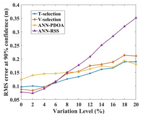
FIGURE 15. RMS error comparison of 90% CDF at different variation level.
