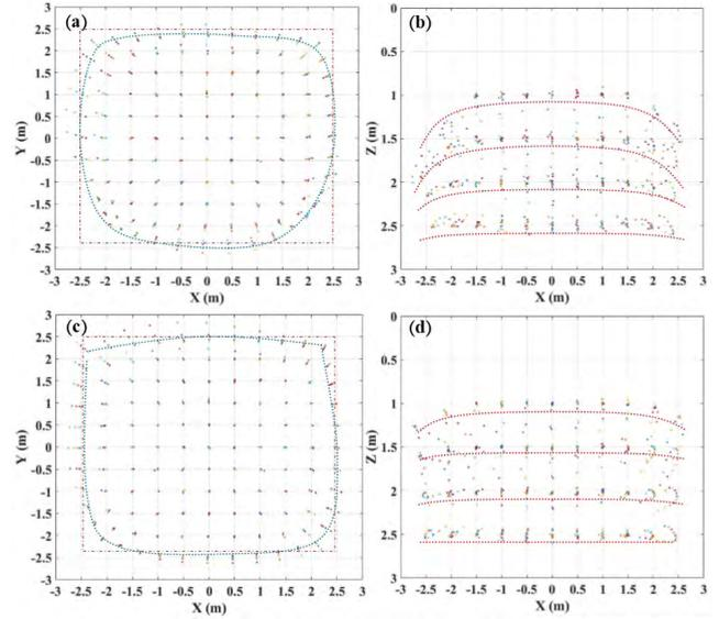
**FIGURE 10.** Estimation results of ANN-PDOA positioning w/wo the pre-training method at 5m by 5m coverage (in (a)&(c) squared boundaries are the ideal testing area, blue curves illustrate the bound of estimated positions; in (b)&(d) the red curves indicate the trend of distortions in X direction at different heights): a) X-Y view of ANN-PDOA w/o pre-training; b) X-Z view of ANN-PDOA w/o pre-training; c) X-Y view of ANN-PDOA w pre-training; d) X-Z view of ANN-PDOA w pre-training.
