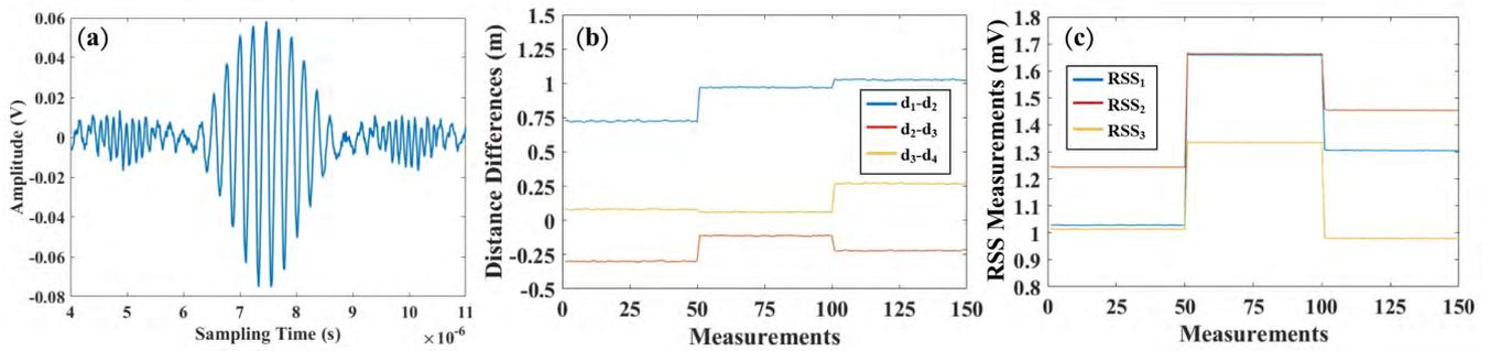
FIGURE 6. Received Waveform and measurements a) Waveform example; b) PDMs of distance differences; c) Intensity based RSSMs.
