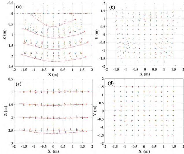
**FIGURE 9.** Simulation on ITD influences to PDOA measurements based positioning system (dashed arrows indicate the trend of distortions in X direction at different heights) a) conventional PDOA positioning results in X-Z view; b) conventional PDOA positioning results in X-Y view; c) ANN-PDOA positioning results in X-Z view d) ANN-PDOA positioning results in X-Y view.
