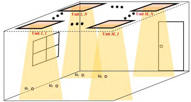
**FIGURE 1.** Indoor VLP system with multiple VLP units.
