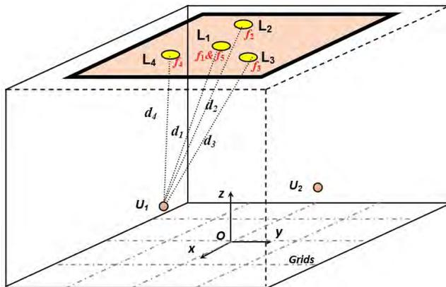
FIGURE 2. System architecture of one VLP unit.
