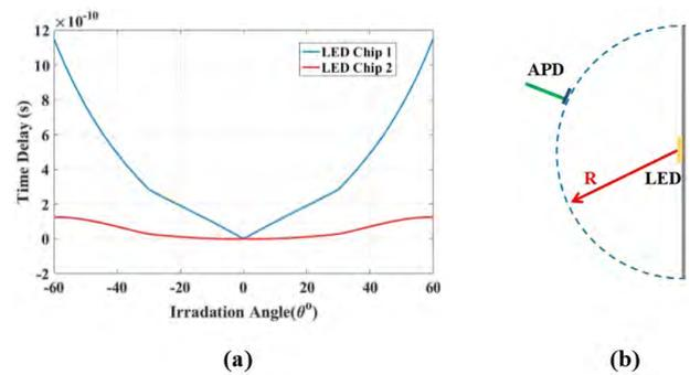
FIGURE 8. Initial time delay distribution of different types of LED chips a) Relationship between irradiation angle and signal time delay; b) illustration of ITD measurements' setup, dashed semicircle have the same distance to the LED.
