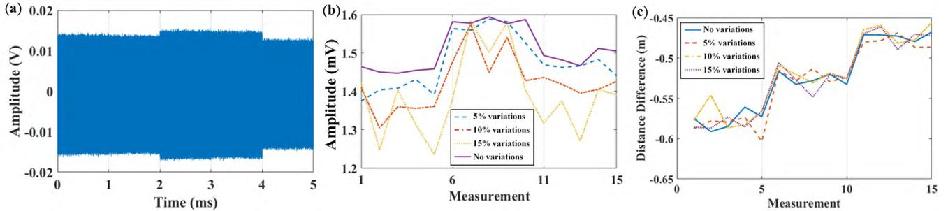
FIGURE 11. Waveforms of different intensity variations a) example of received signal under 15% intensity variations; b) RSSMs under different variation levels; c) PDMs under different variation levels.
