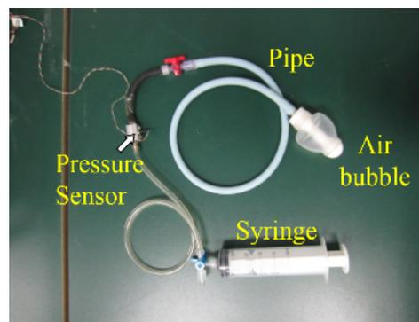
**FIGURE 1.** Picture of the intravaginal pressure acquisition device, consists of an air bubble, a pipe, a pressure sensor, and a syringe.
