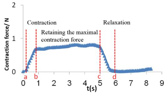
**FIGURE 3.** A typical curve of slow-contraction including the contraction period (from point a to b), retaining period (from point b to c) and relaxing period (from point c to d).
