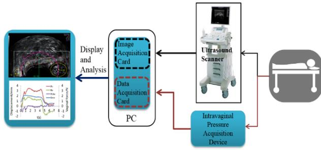
**FIGURE 2.** System diagram to simultaneously collect the intravaginal pressure and ultrasound images of levator ani muscles during active contraction and relaxation by the subject.
