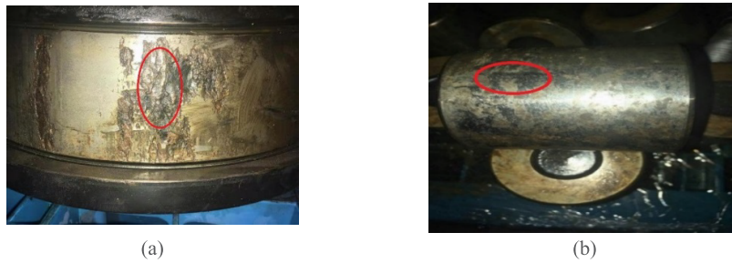
FIGURE 7. Bearing inner ring and rolling element failure diagram. (a) Bearing inner ring peeling off; (b) bearing rolling body pitting.
