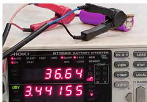
FIGURE 13. Results of internal resistance measurement. T = 15°C.
