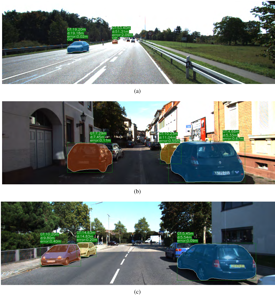
FIGURE 12. Distance experimental results on KITTI dataset.
