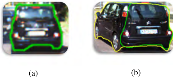
FIGURE 6. Outline map of target vehicle candidate area, (a) Mask outline of the Front vehicle. (b) Mask outline of Sideway vehicle.
