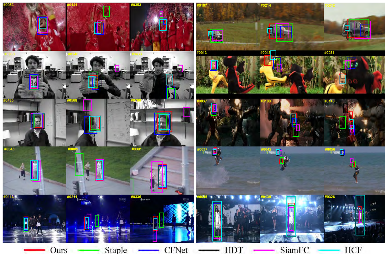
FIGURE 11. The display of tracking results. We select the partial tracking results of Staple, CFNet, HDT, SiamFC, HCF and proposed algorithm in 10 challenging image sequences (from left to right, top to bottom, respectively, are soccer, carscale, cliffbar, dragonbaby, fleetface, ironman, jogging-2, kitesurf, skating1, singer1).
