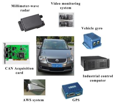
FIGURE 1. Components of the test vehicle platform.
