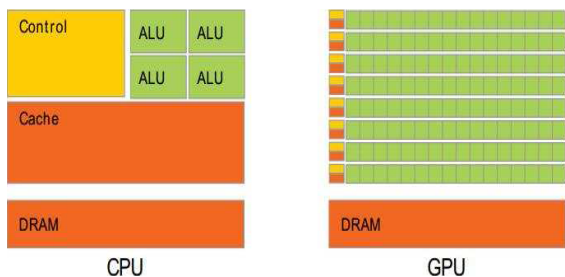
FIGURE 5. The native difference between CPU and GPU architectures.
