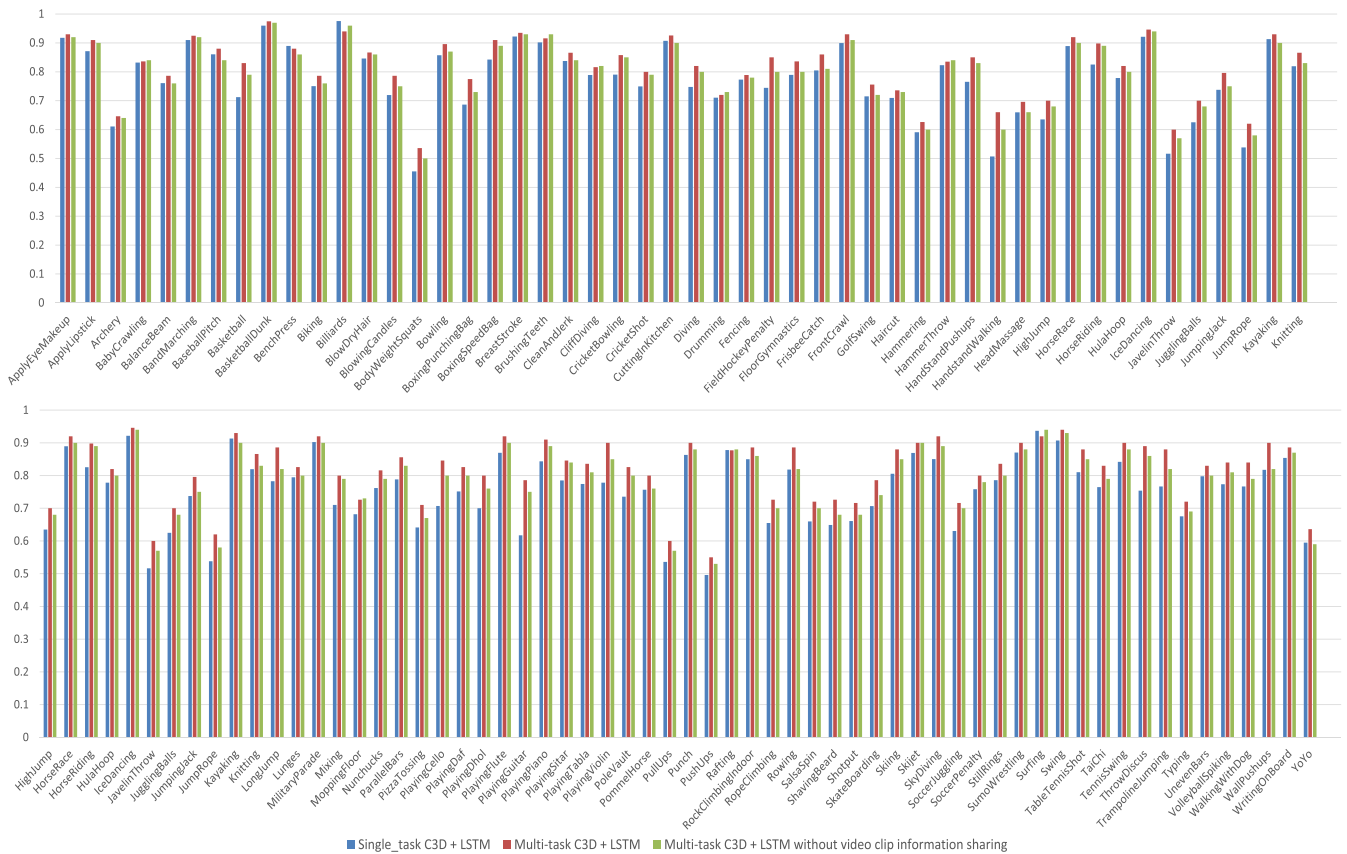
FIGURE 6. Classification accuracy of each category on UCF101 dataset. Blue indicates the classification accuracy of single-task C3D + LSTM and red indicates the classification accuracy of multi-task C3D + LSTM. Meanwhile, green indicates the classification accuracy of the multi-task C3D + LSTM without video clip information sharing.
