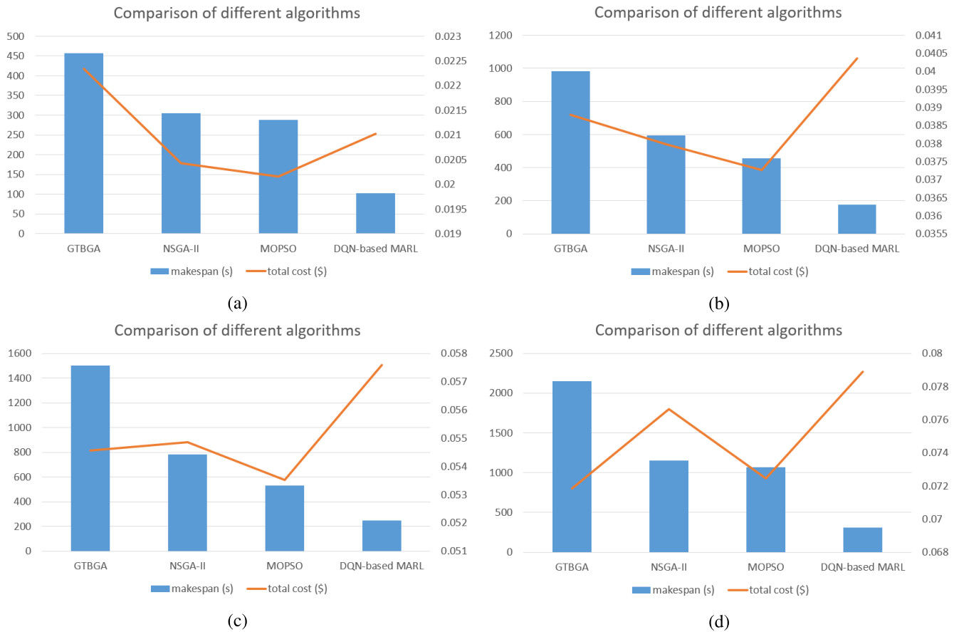
FIGURE 5. Illustration of comparisons of baseline algorithms and DQN-based MARL method with four different task sizes. (a) 138; (b) 252; (c) 358 and (d) 497.
