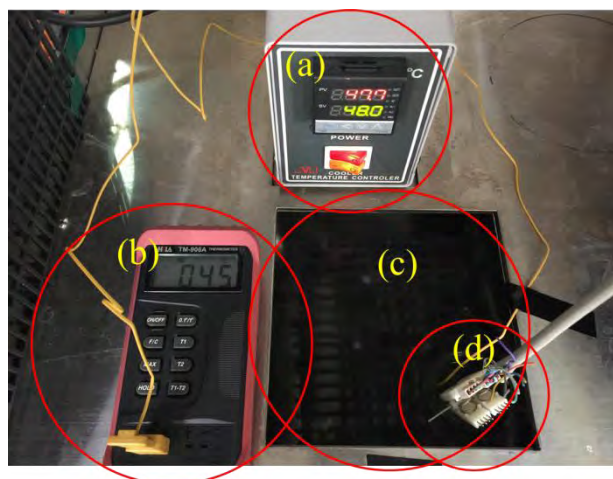
FIGURE 5. The setting of thermostatic water bath for temperature effects. (a) The temperatures controller, (b) digital thermometer, (c) the water bath, and (d) the biosensor.
