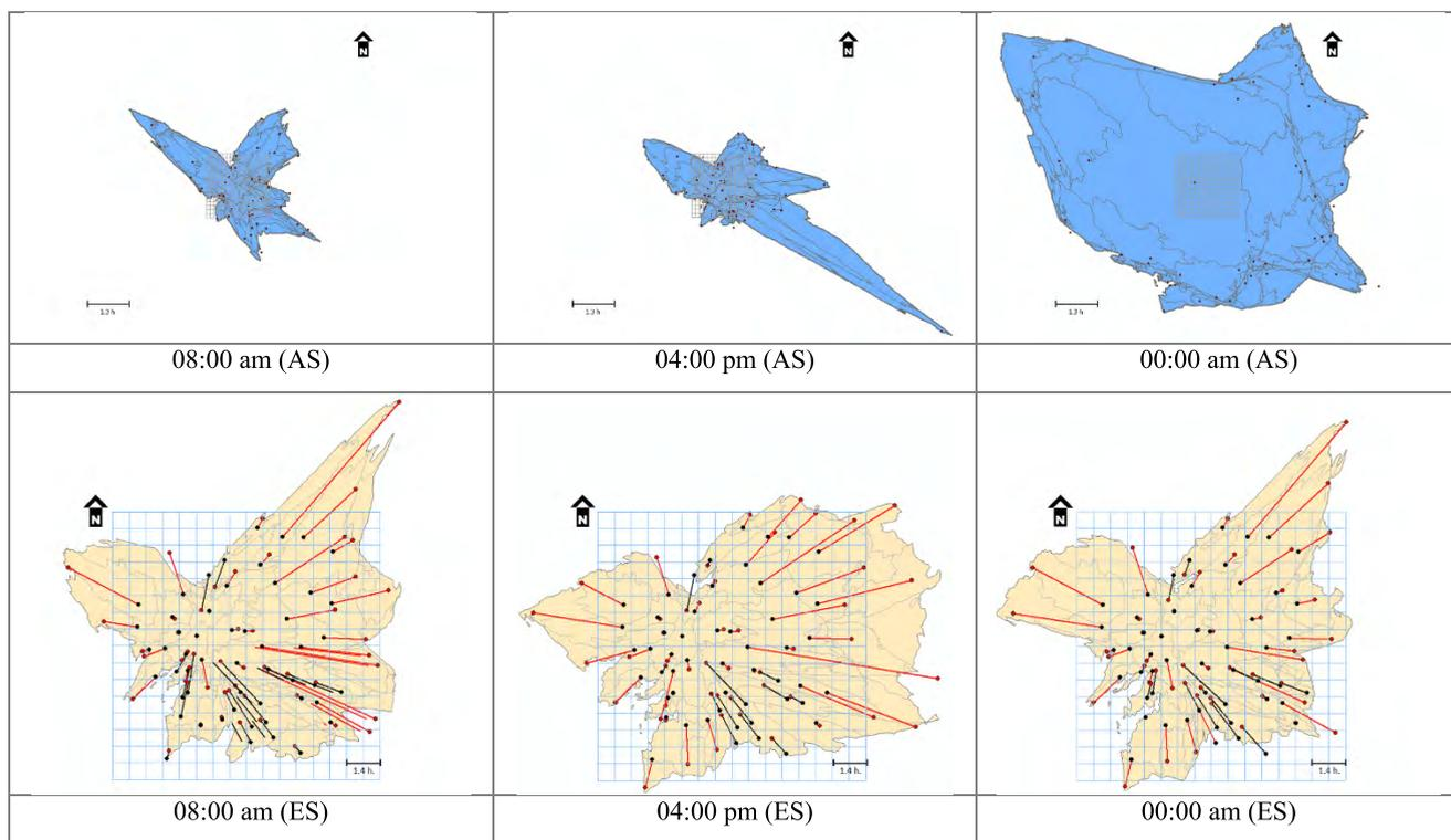
FIGURE 14. Time-distorted maps at different time periods. In the ET scenario, black vectors indicate shrinkage effect, while red ones indicate stretching effect.
