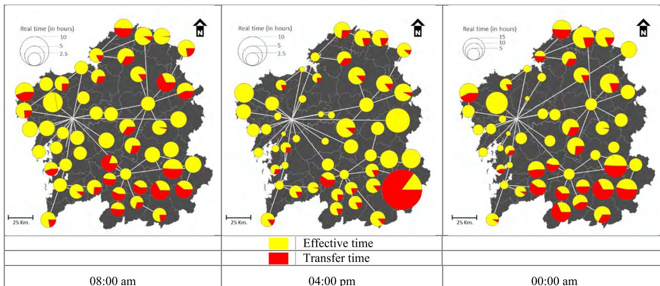
**FIGURE 6.** Time required for traveling from the central node to the other ones at different time periods. The circle size is related to the total travel time that is required (AS). The yellow color shows the effective travel time (ES), and red color shows the transfer time required between transport modes when appropriate.
