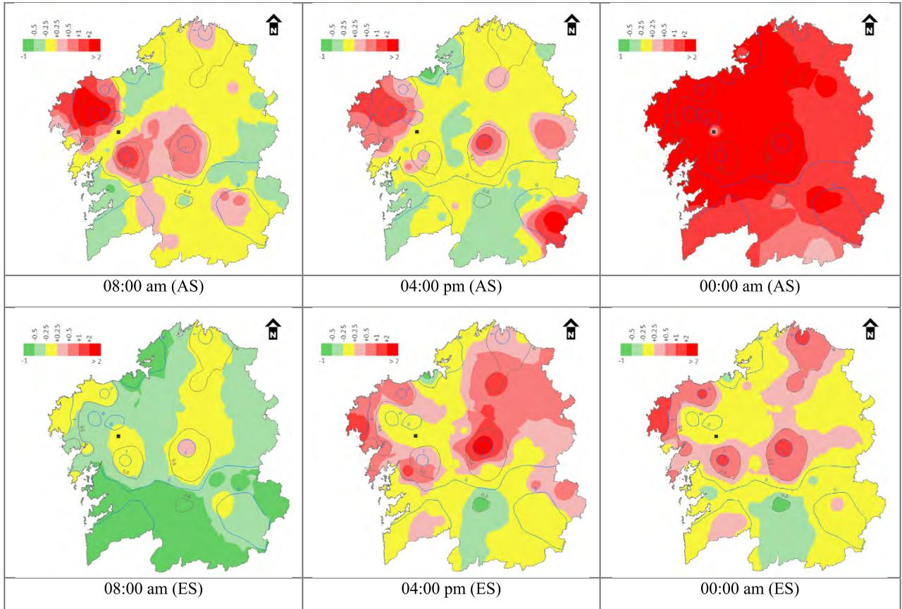
**FIGURE 11.** Distortion rate of the whole region with respect to the central node at different time periods. Results for both scenarios are represented. Contour lines represent distortion rates, whose time value (in minutes) is shown in labels.
