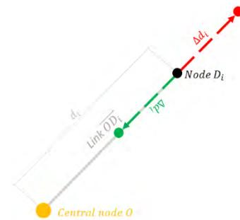
**FIGURE 4.** Parameters for the estimation of distortion rate ( $R_i$ ) based on the Euclidean distance ( $d_i$ ) and the distortion of this distance ( $\pm \Delta d_i$ ). Final node location will be closer/farther to/from the central node depending on the relation between  $V_i$  and  $V_{ref}$ .
