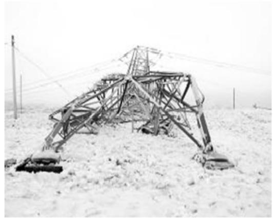
**FIGURE 2.** Transmission line ice accidents [6,7].
