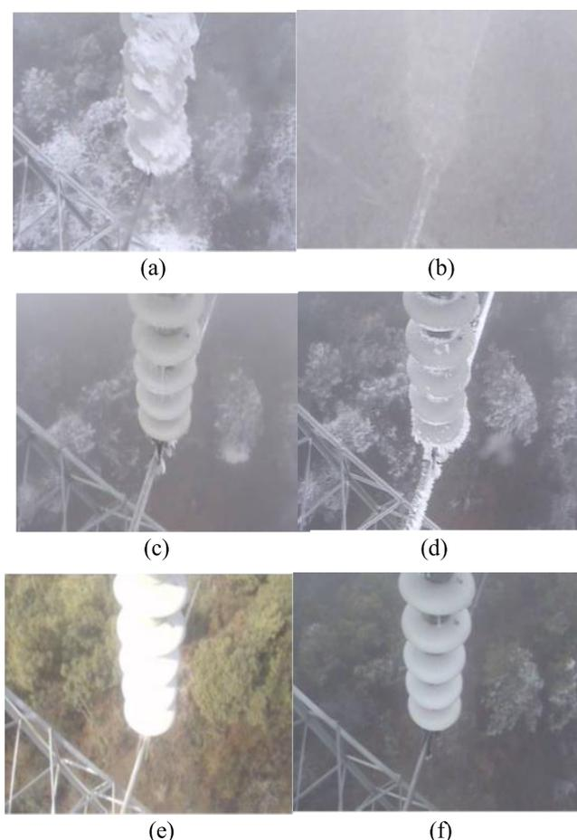
**FIGURE 10.** Transmission line ice coating grade. (a) Grade 0. (b) Grade1. (c) Grade2. (d) Grade 3. (e) Grade 4. (f) Grade 5.
