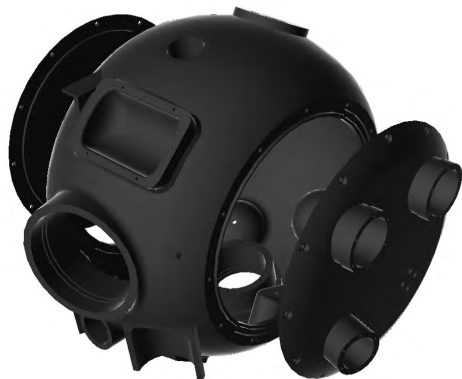
FIGURE 3. Exploded view of robot aluminum external hull and side plates for sealing the watertight hull and fixing manifolds.
