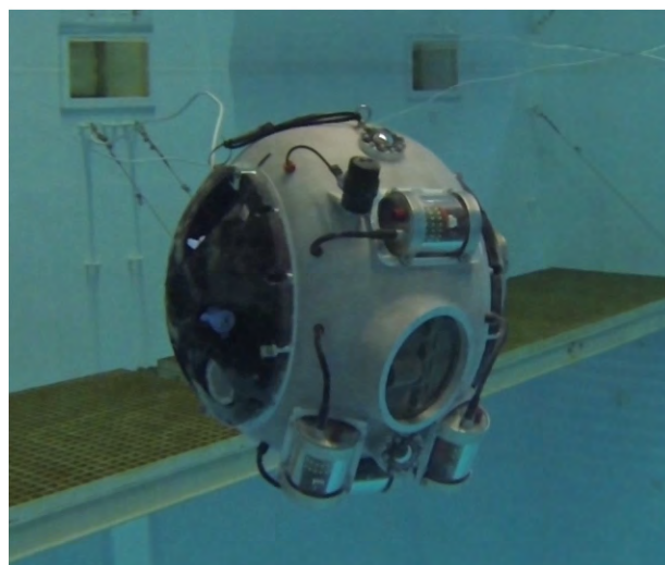
FIGURE 1. Proposed spherical underwater vehicle prototype during pool tests.
