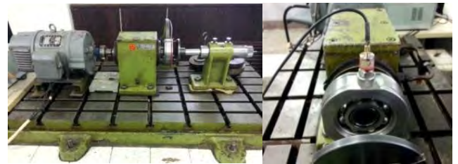
FIGURE 18. Bearing experiment platform for fault diagnosis.
