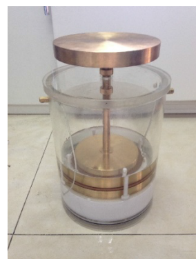
FIGURE 5. Three electrodes for FDS experiments.
