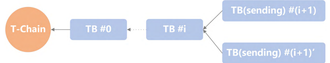
FIGURE 4. A fork occurs when two (or more) signed transaction blocks reference the same previous block. Older transaction blocks are on the left; newer blocks are on the right.
