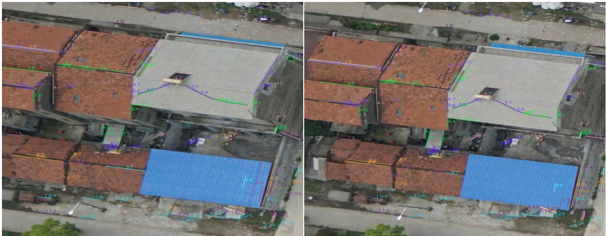
FIGURE 13. Line matches of (c) from the UAV image: Extracted line segments: 855, 790. Total matches: 136. Correct matches: 135.
