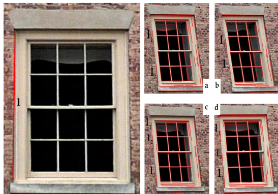
FIGURE 4. Structure line segments: The left-hand image contains a line segment that is not broken. The a, b, c and d fragments show several fragments due to changes in scale, viewpoint and illumination. Matching these fragments in different views is difficult due to the lack of exact endpoints. For example, l_i ( i = 1, 2 or 3 ) in a, b, c and d represent parts of line segment l.
