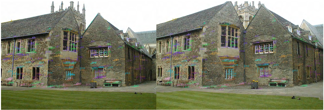
FIGURE 8. Line matches of Merton: Extracted line segments: 786, 757. Total matches: 331. Correct matches: 330.
