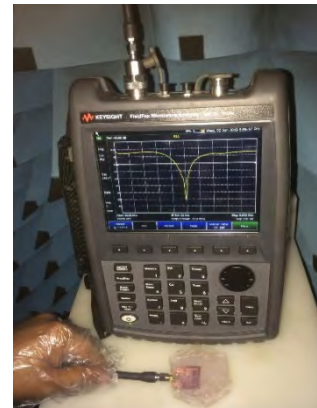
FIGURE 9. Measurement of S_{11} in phantom mimicking muscle gel of an ICCP antenna.
