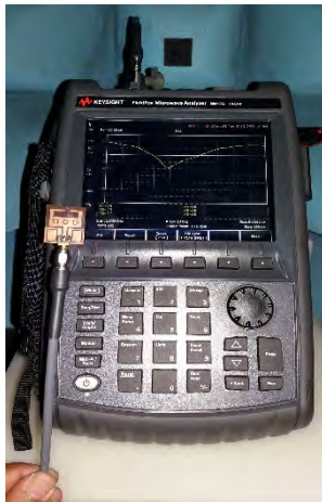
FIGURE 7. Measurement of S_{11} in the free space of an ICCP antenna.
