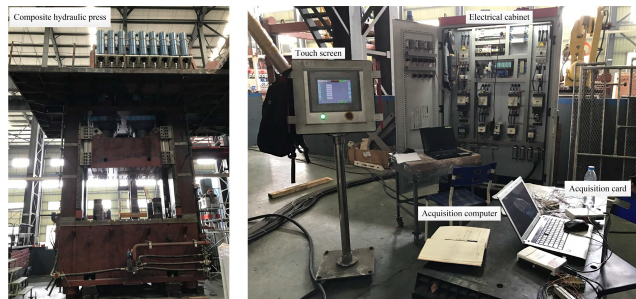
FIGURE 18. Mobile crossbeam variable-speed falling system experiment platform.
