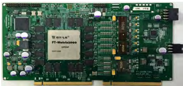
FIGURE 14. The testing board for CPU accelerator.
