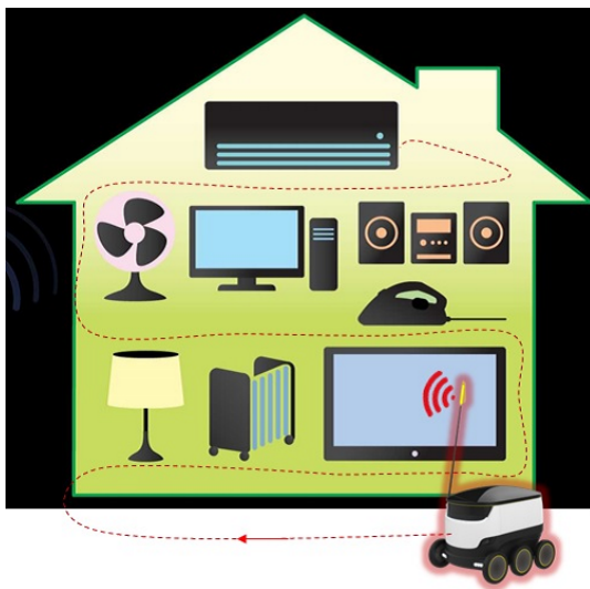
FIGURE 5. A wireless mobile unit going around to collect RSSIs from IoT devices.
