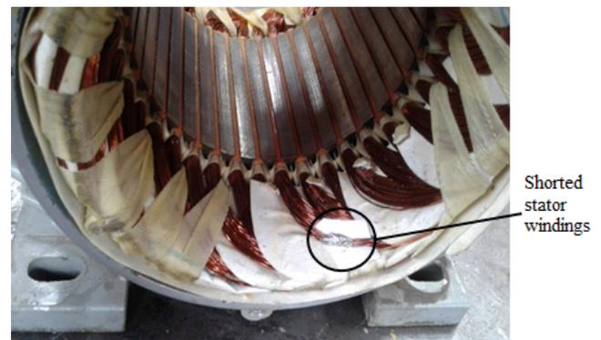
**FIGURE 6.** Experimental implementation of stator winding inter-turn short-circuit fault.
