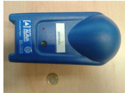
FIGURE 4. EME Spy 121 personal dosimeter used for the campaign of measurements within the buses.
