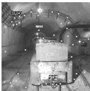
FIGURE 6. Feature points of extracted locomotive image.
