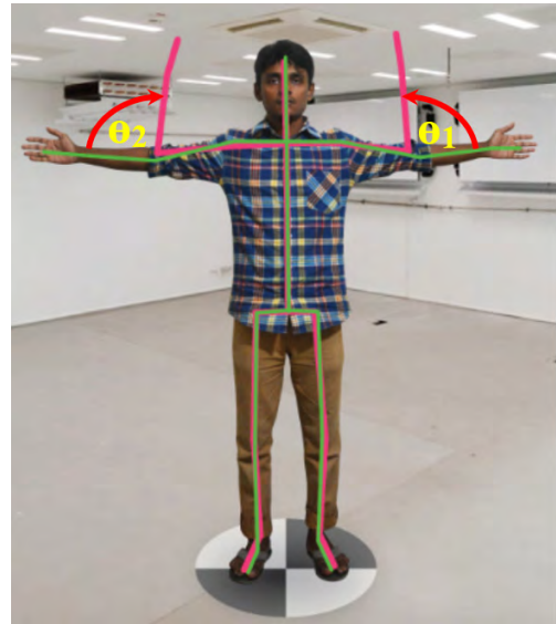
FIGURE 8. Forward kinematic data obtained from gesture tracking sensor shown in Figure 7 is applied to deduce inverse kinematic principles in order to follow the virtual occupational therapist in an augmented reality view.
