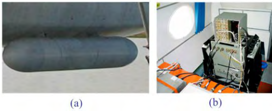
FIGURE 7. Airborne SAR system, (a) antenna pod, (b) radar hardware system.
