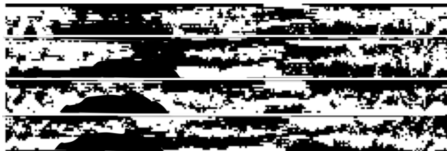
FIGURE 11. The most relevant features selected from each of the four QQC encoding images. Top row image represents the real part. Second, third and fourth rows represent the imaginary part. White pixels represent features selected.
