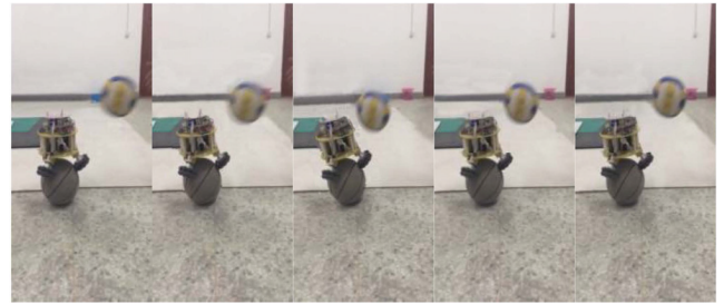
FIGURE 11. A series of picture of the ballbot smashed by volleyball.
