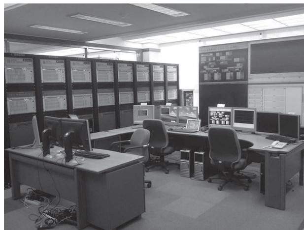
**FIGURE 10.** RTDS system in EHV power transmission company, CSG.
