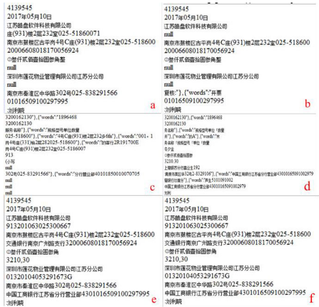
FIGURE 14. Comparison of identification results on a scanned invoice.
